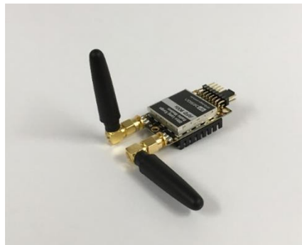
Figure 8-1: Antenna configuration to achieve polarisation diversity
