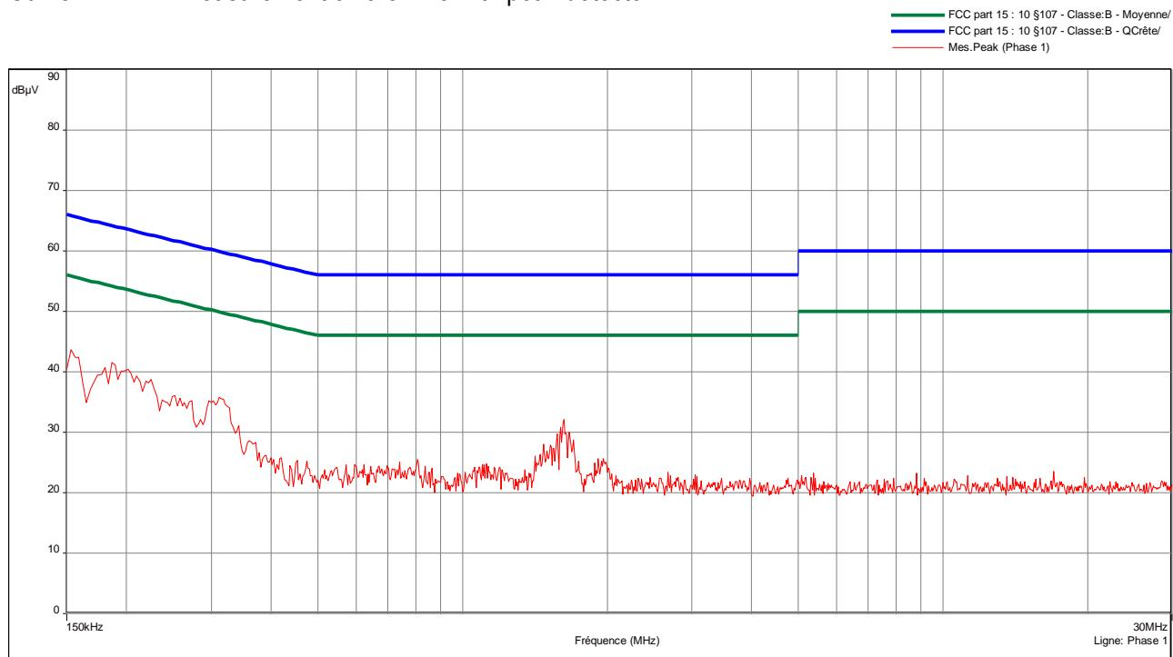
**Measurement on the mains power supply: Mode 2 WIFI in RX mode**
