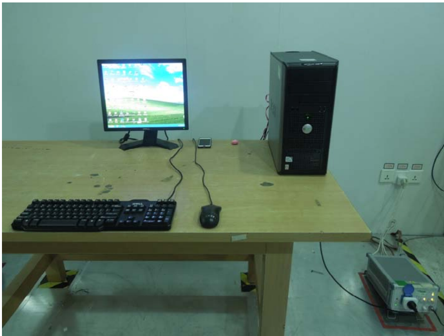
Photo of Setup for Conducted Emission
