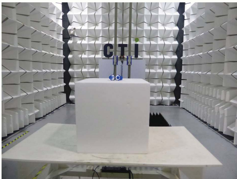
Radiated spurious emission Test Setup-2(Above 1GHz)
