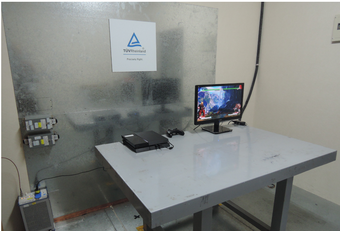
Photograph 8: Set-up for Mains Conducted testing (Front view)
