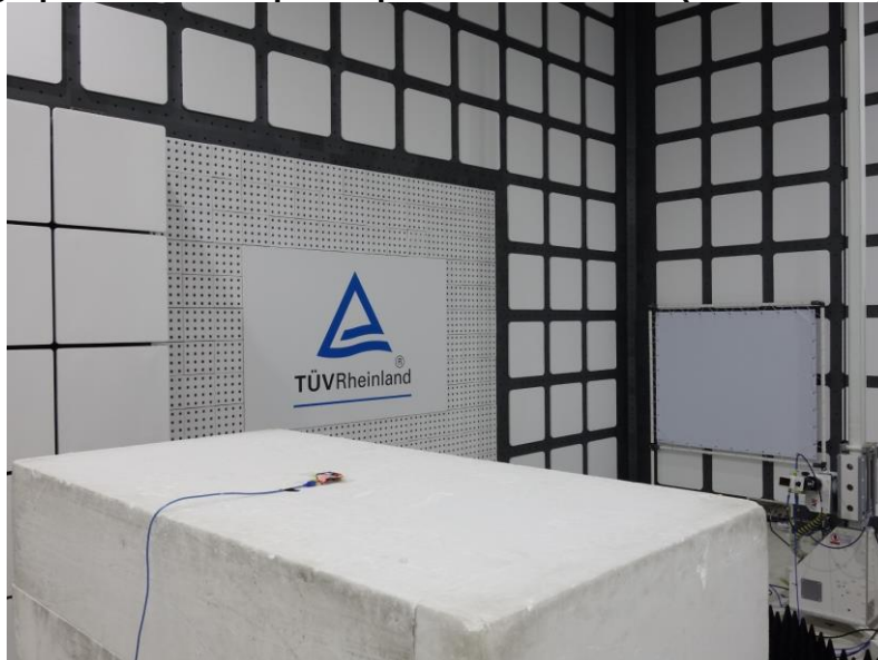
Photograph 6: Test Setup for Spurious Emissions (Back View 4)
