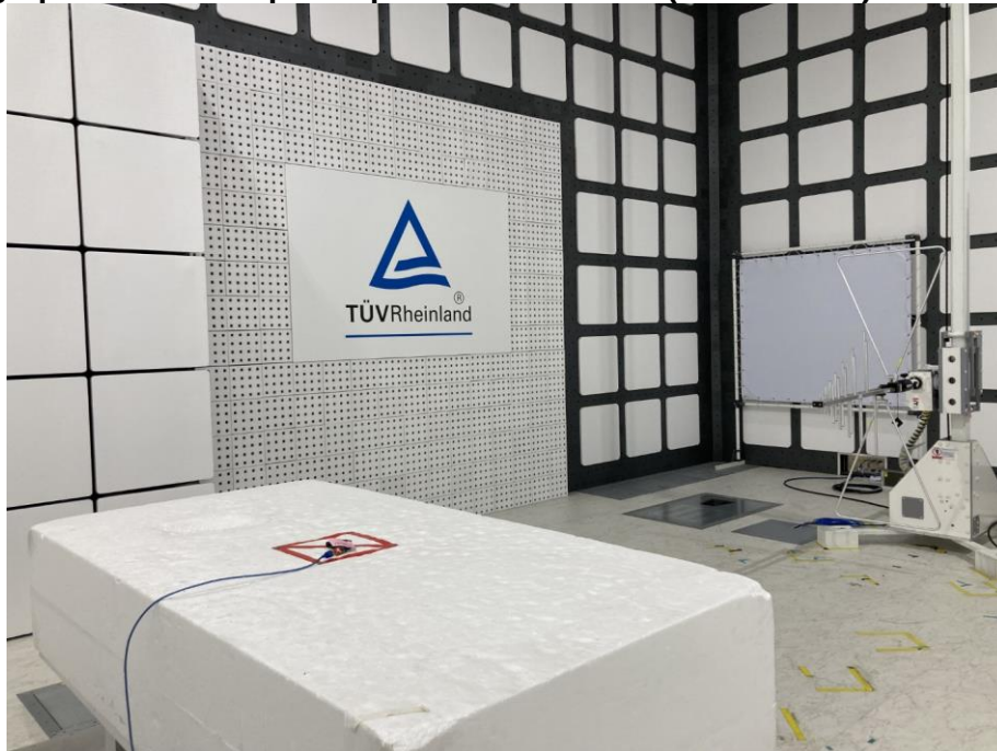
Photograph 4: Test Setup for Spurious Emissions (Back View 2)
