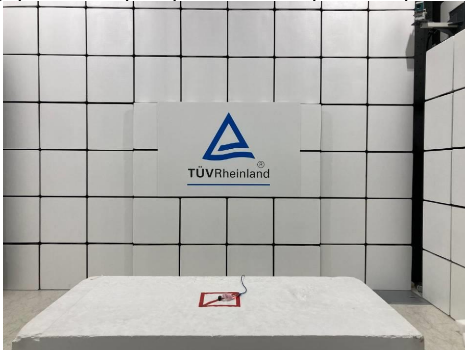
Photograph 2: Test Setup for Spurious Emissions (Front View 2)
