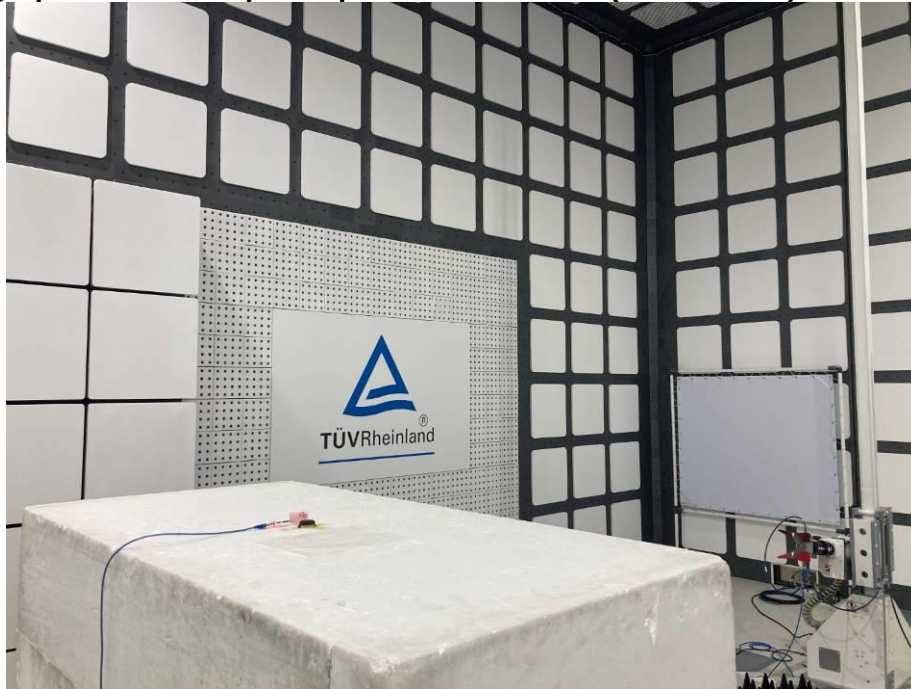
Photograph 6: Test Setup for Spurious Emissions (Back View 4)
