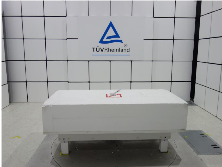
Photograph 1: Test Setup for Spurious Emissions (Front View 1)
