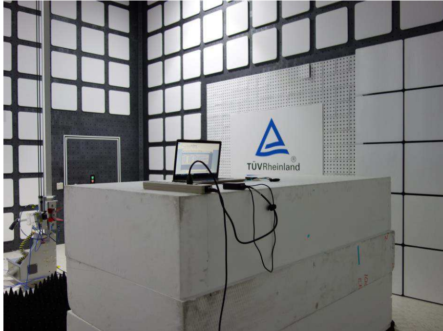
Photograph 3: Set-up for Spurious Emissions (Back View 1)
