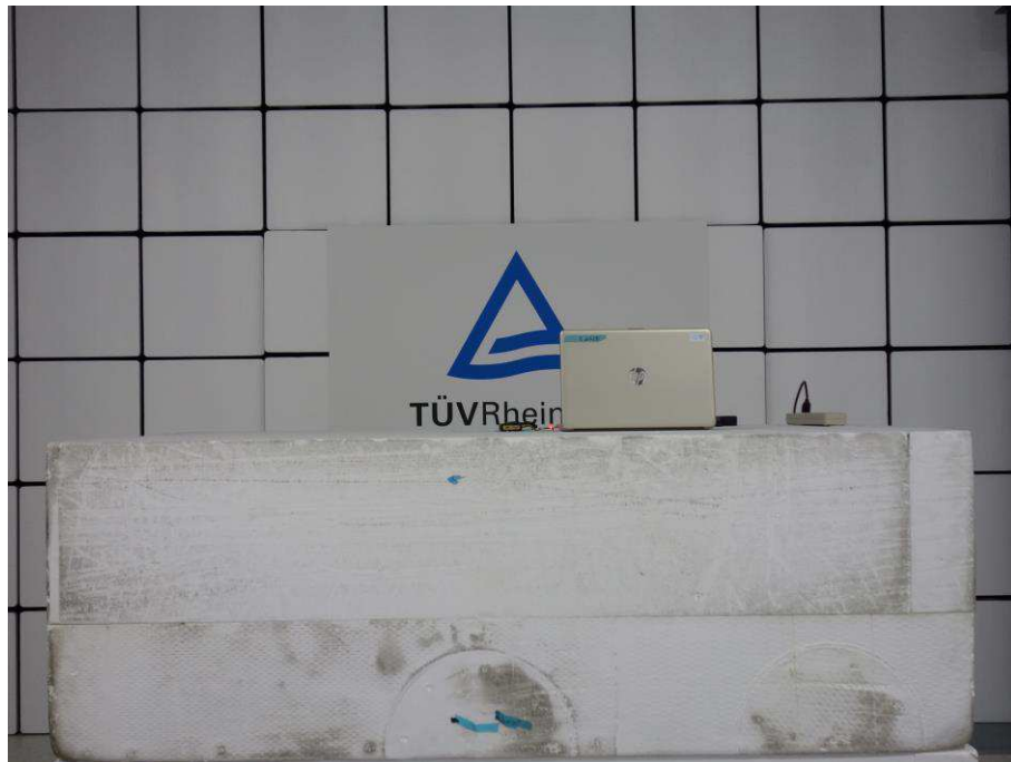
Photograph 2: Set-up for Spurious Emissions (Front View 2)
