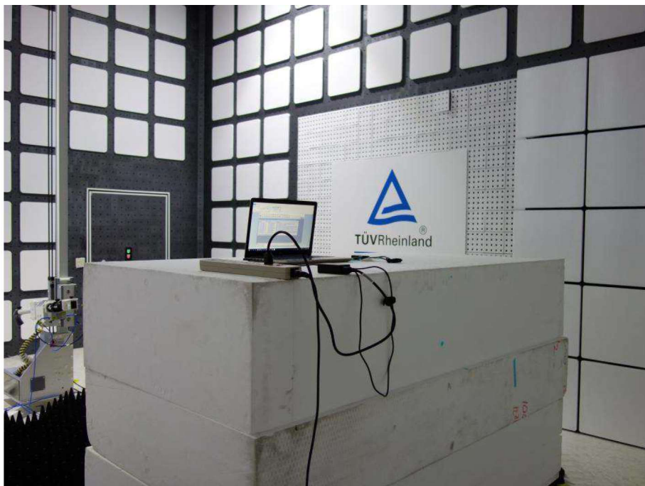
Photograph 4: Set-up for Spurious Emissions (Back View 2)
