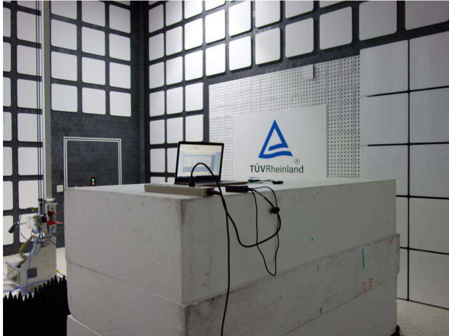
Photograph 3: Set-up for Spurious Emissions (Back View 1)
