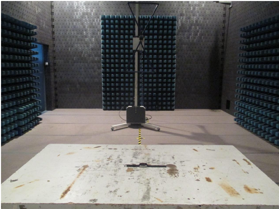
Radiated Emission Test setup photos
