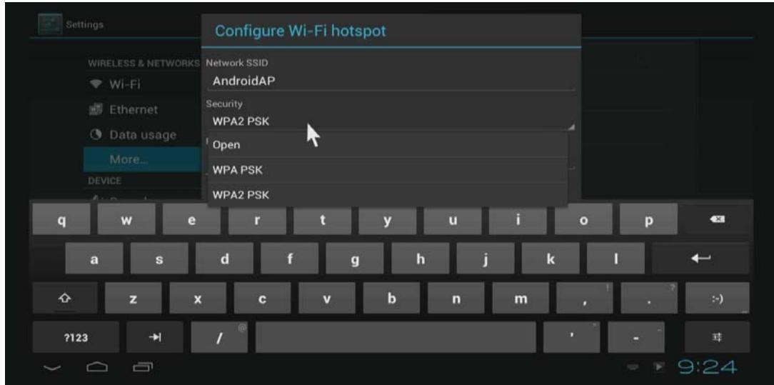
Note: WiFi and hotspot connection can not be applied at same time. Disconnect WiFi and connect Ethernet while using hotspot function.
