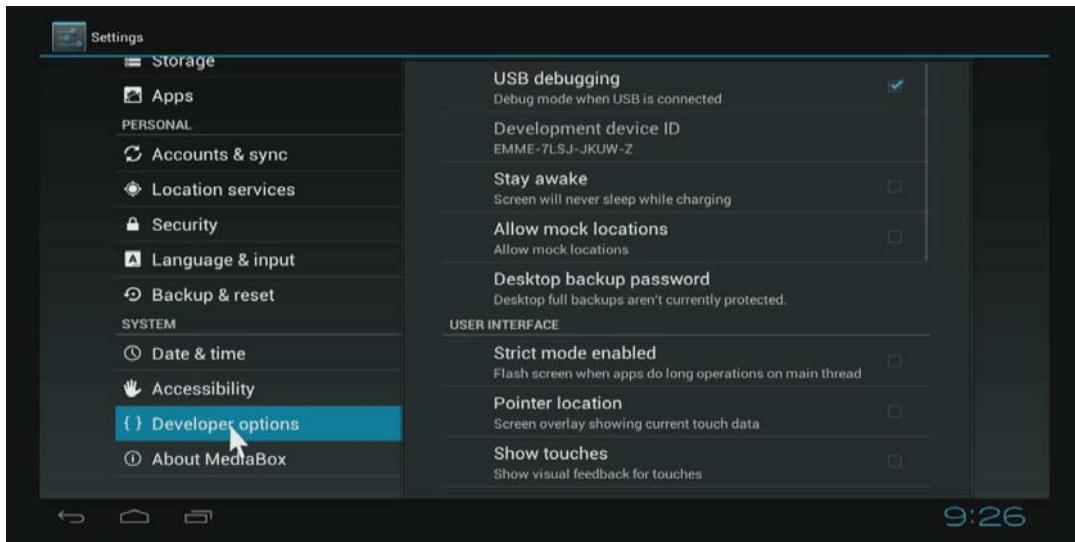
If user want to do some debugging on box by ADB, enable USB debugging, you will get ADB function by Ethernet or WiFi network.
