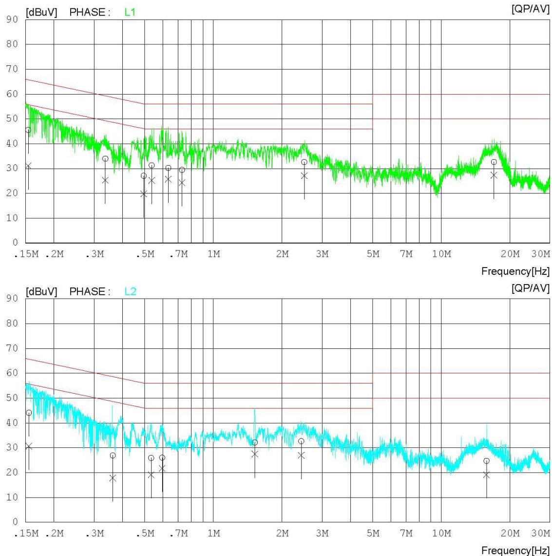
**AC Line Conducted Emissions (Data List)****Results of Conducted Emission**
