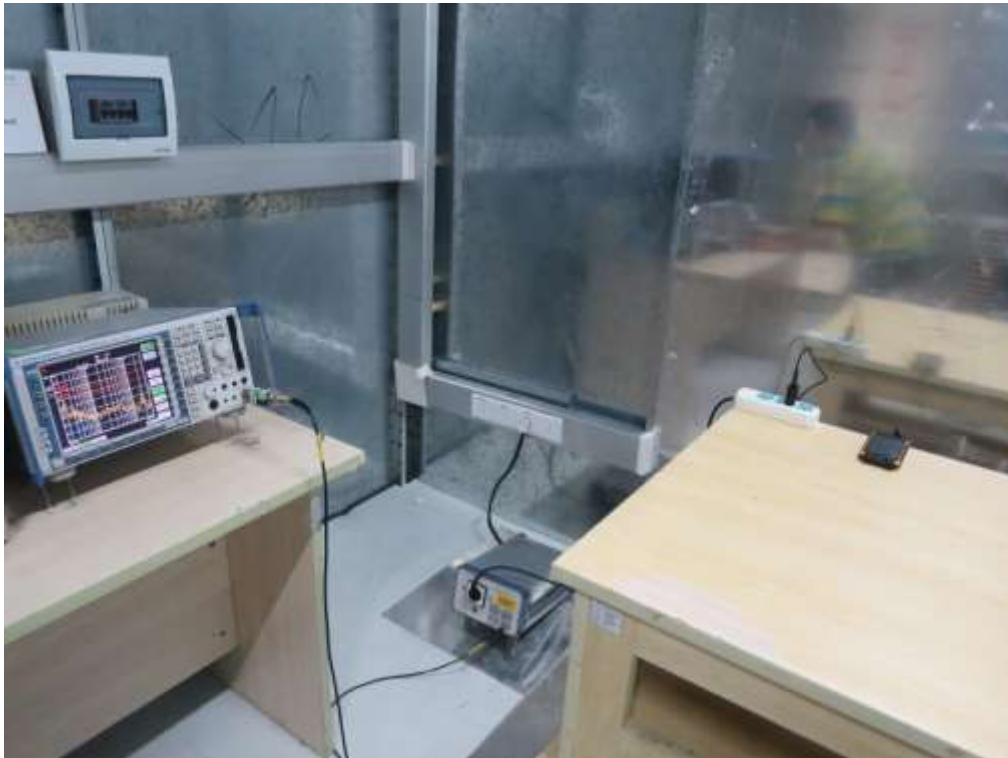
FCC RADIATED EMISSION TEST SETUP
