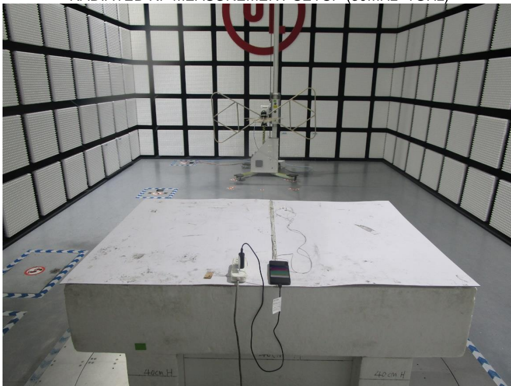
RADIATED RF MEASUREMENT SETUP (Below 30MHz)
