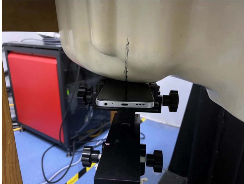
Head Right Cheek Setup Photo (0mm)
