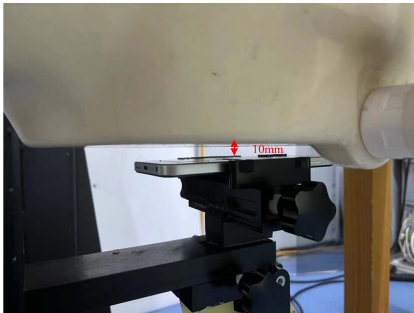
Body (Wron)Back Setup Photo (10mm)
