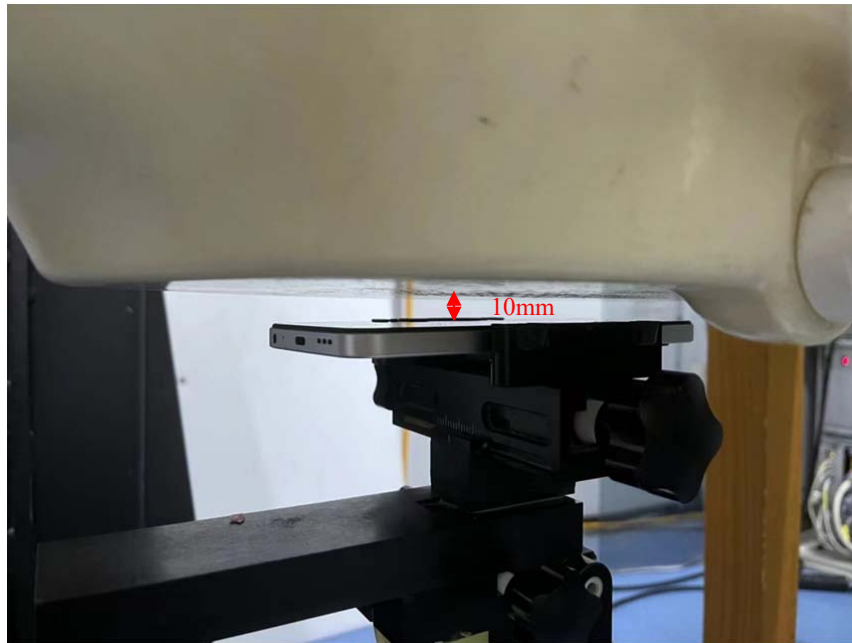
Body (Wron)Front Setup Photo (10mm)
