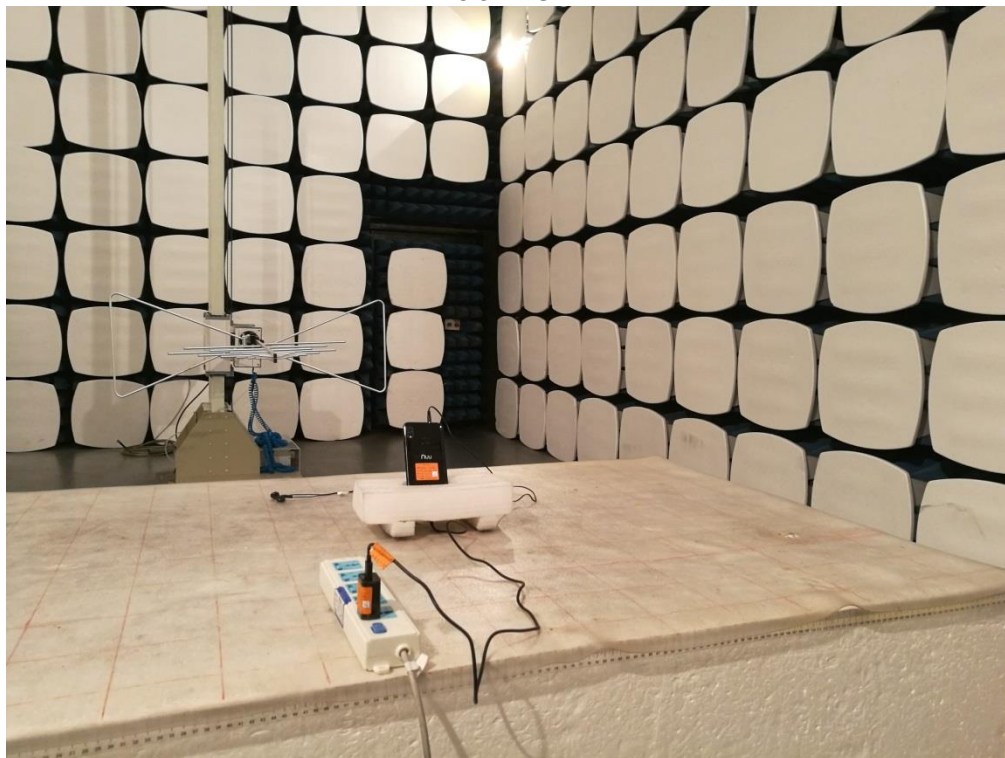
Radiated Spurious Emission Below 1GHz
