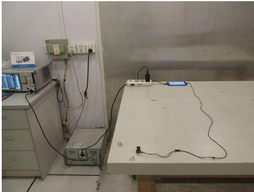
CONDUCTED EMISSION TEST
