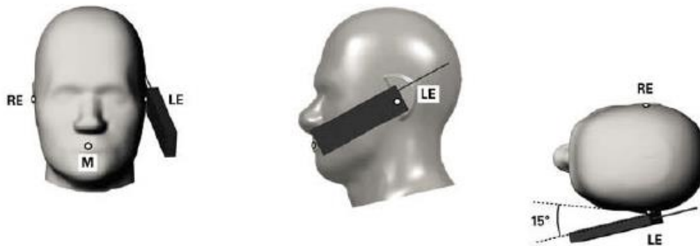
Fig.11.4 Illustration for Tilted Position
