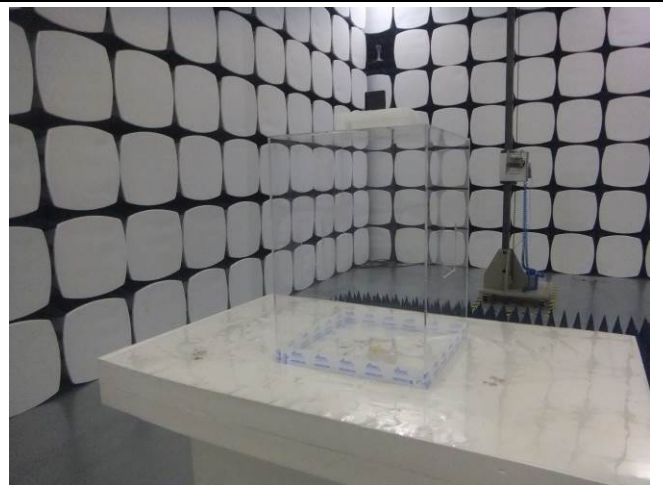
Radiated Spurious Emissions Test Setup Above 1GHz
