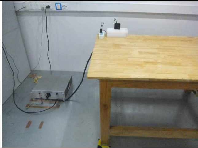
Conducted Emissions Test Setup Front View
