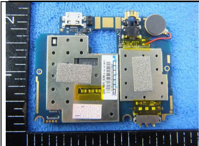
Mainbard with Shielding - Rear View
