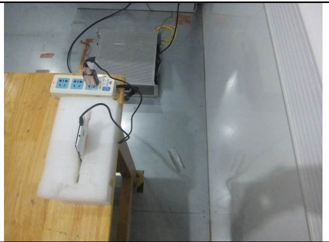
Conducted Emissions Test Setup Side View
