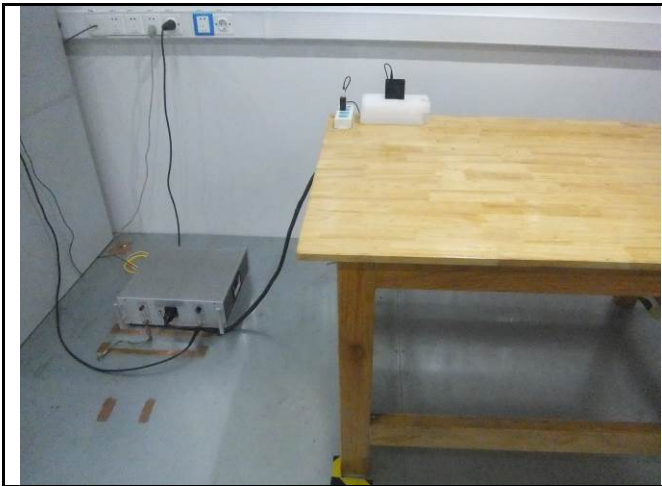
Conducted Emissions Test Setup Front View
