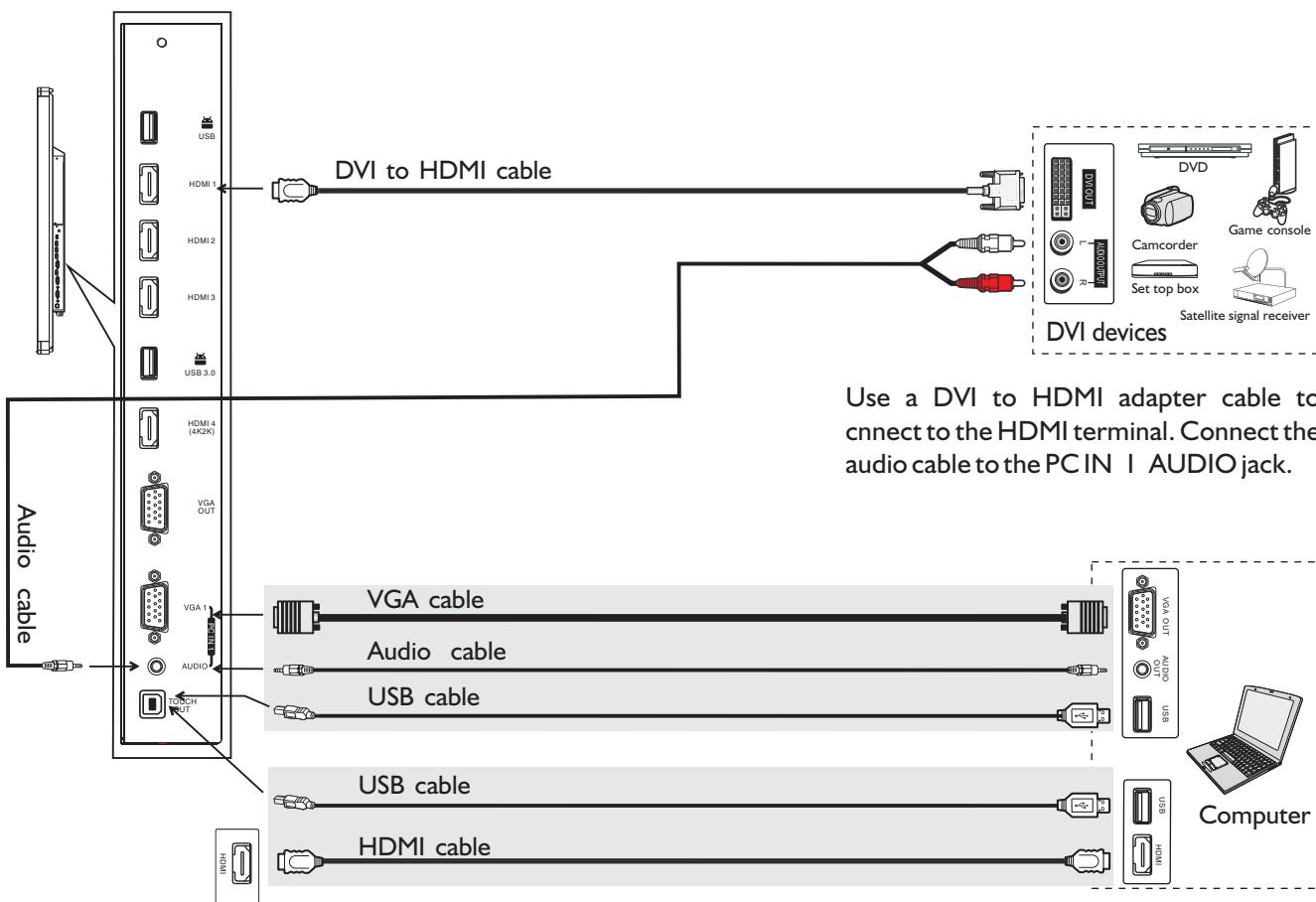
Connect PC with VGA cable or HDMI cable.
