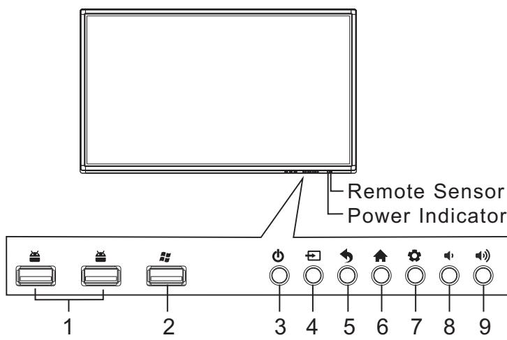
1. : USB standard interface of the IFP (Android system), enable connection to USB2.0 standard devices.
