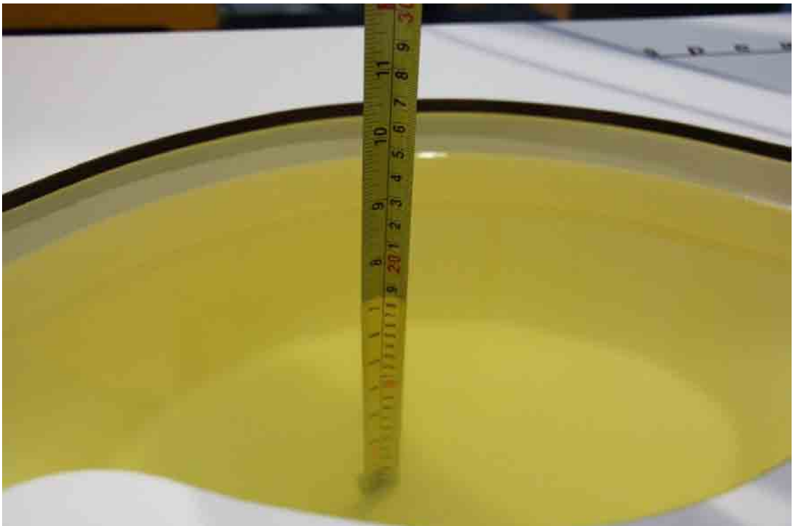
Picture 7-8 Liquid depth in the Flat Phantom (2450MHz)
