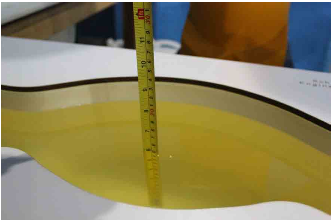
Picture 7-4 Liquid depth in the Flat Phantom (1750MHz)
