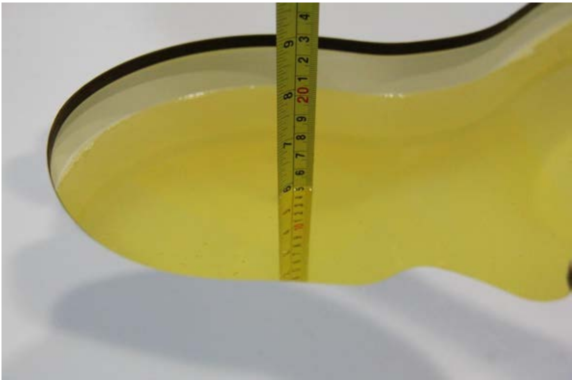
Picture 7-9 Liquid depth in the Head Phantom (2450MHz)
