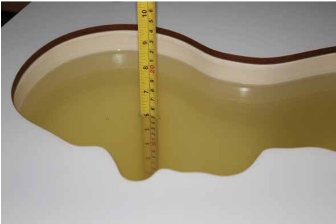
Picture 7-3 Liquid depth in the Head Phantom (1750 MHz)
