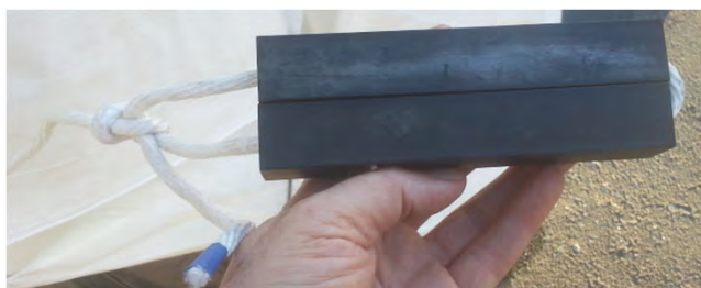
Fig 1: End weighted with resilient blocks, to prevent radome damage.
