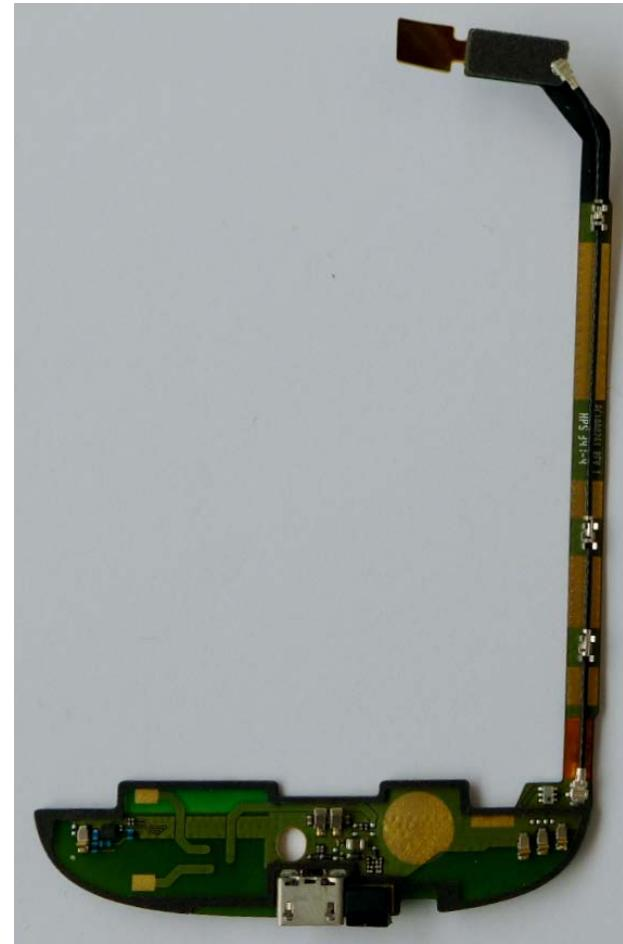
Front display components attached to the flex. Flex can't be removed. No removable shields
