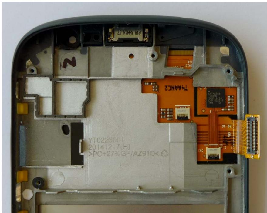
Electronic paper back display. No PCB and no removable shields
