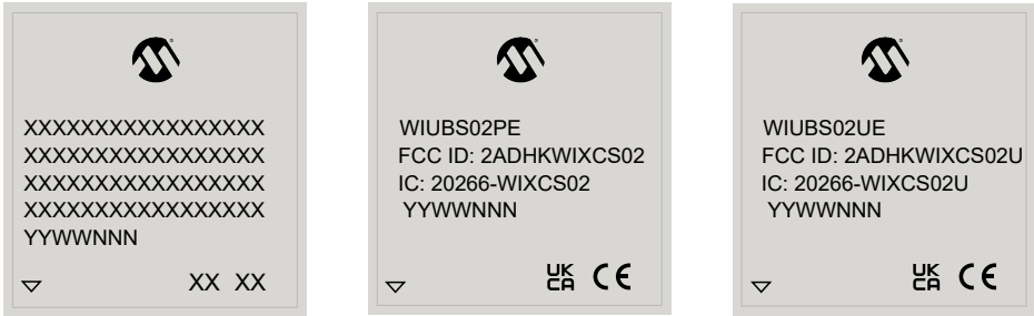
Figure 4-1. WILCS02 Module Packaging Marking
