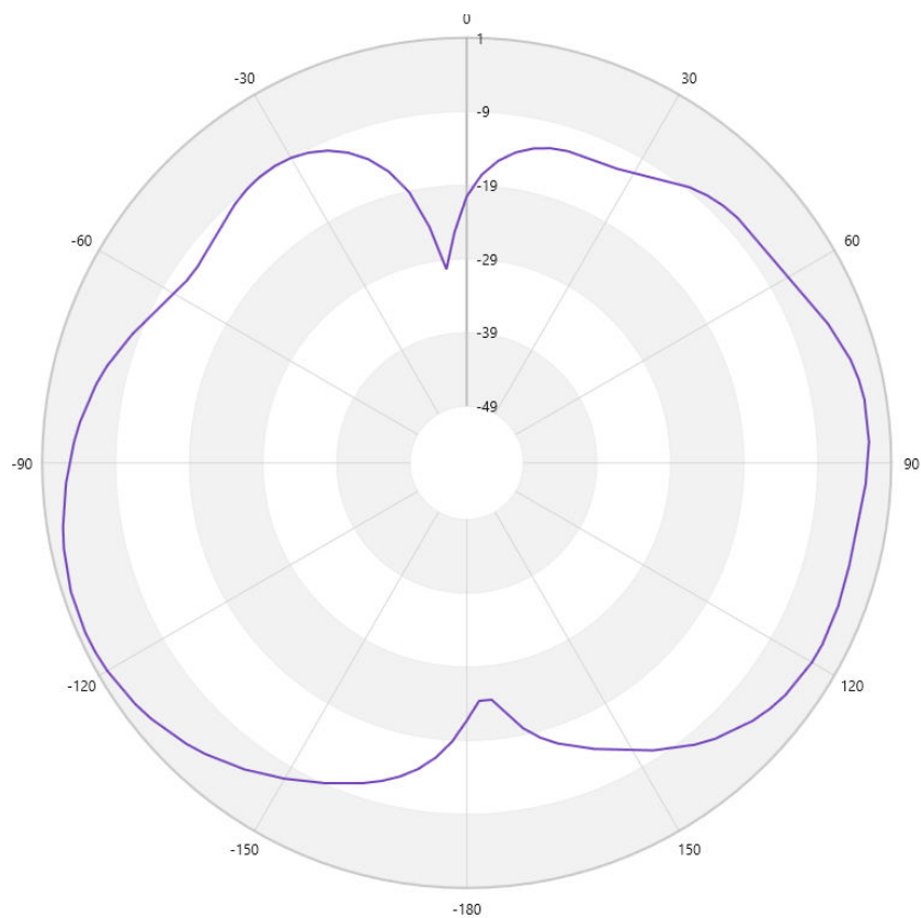
Figure 2-13. Antenna Radiation Pattern when \Phi = 90^\circ
