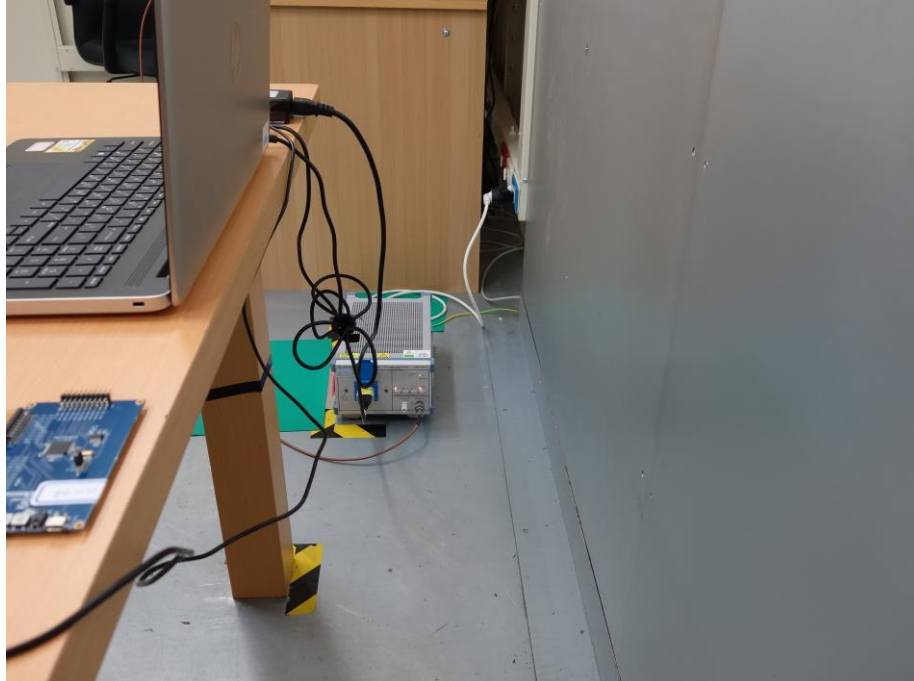
Photograph 16: Test Setup for Mains Conducted Emissions (Back View, WiFi)
