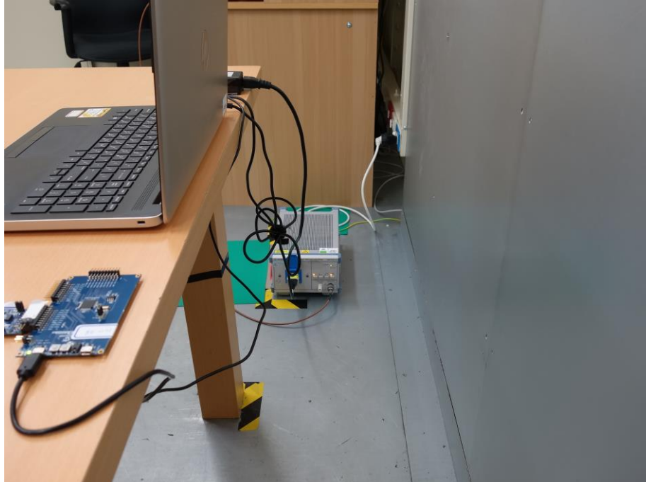
Photograph 32: Test Setup for Mains Conducted Emissions (Back View, WiFi)
