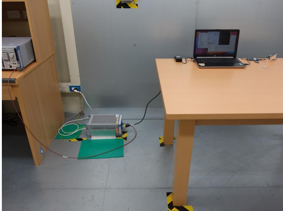
Photograph 8: Test Setup for Mains Conducted Emissions (Back View, BLE)
