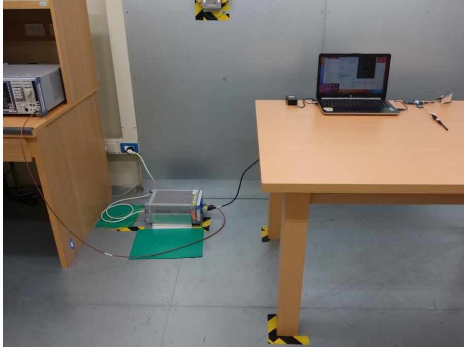
Photograph 23: Test Setup for Mains Conducted Emissions (Front View, BLE)
