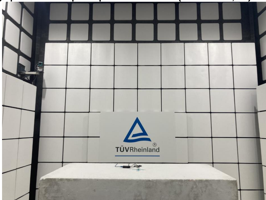
Photograph 2: Test Setup for Spurious Emissions (Front View 2, BT)
