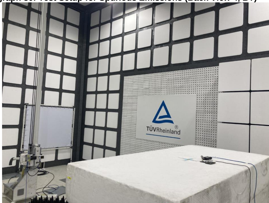
Photograph 30: Test Setup for Spurious Emissions (Back View 4, BT)
