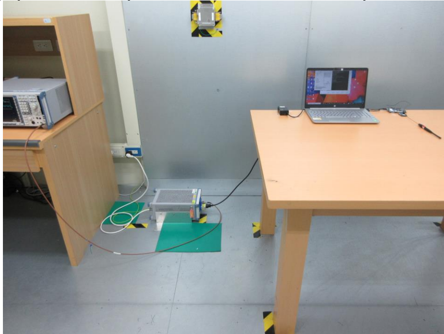
Photograph 71: Test Setup for Mains Conducted Emissions (Front View, WiFi)
