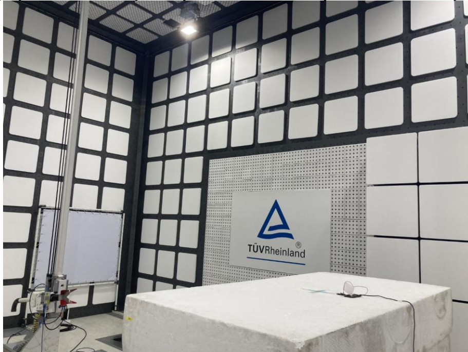
Photograph 45: Test Setup for Spurious Emissions (Back View 3, WiFi)
