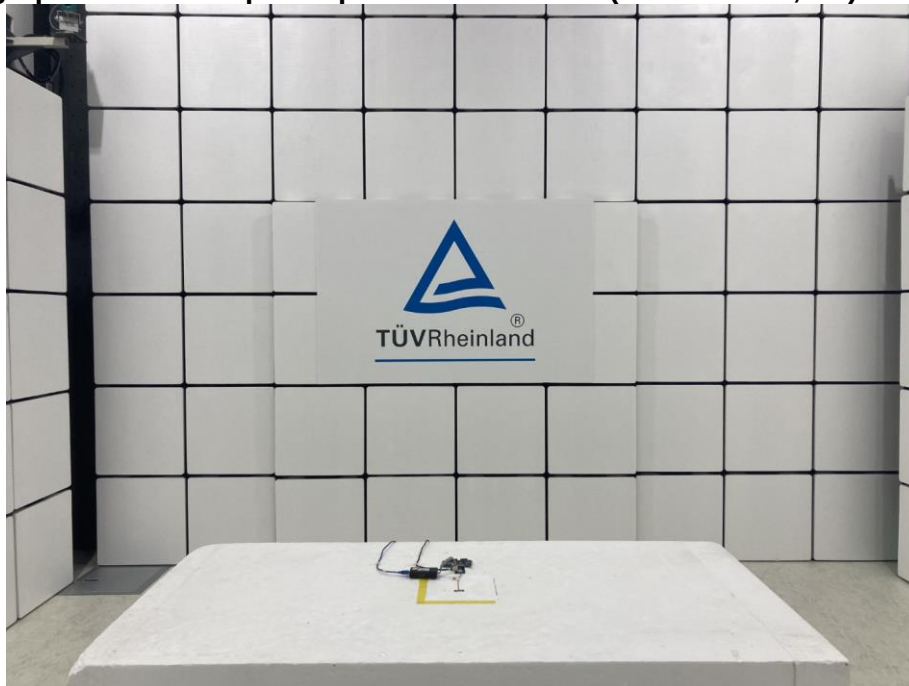
Photograph 1: Test Setup for Spurious Emissions (Front View 1, BT)
