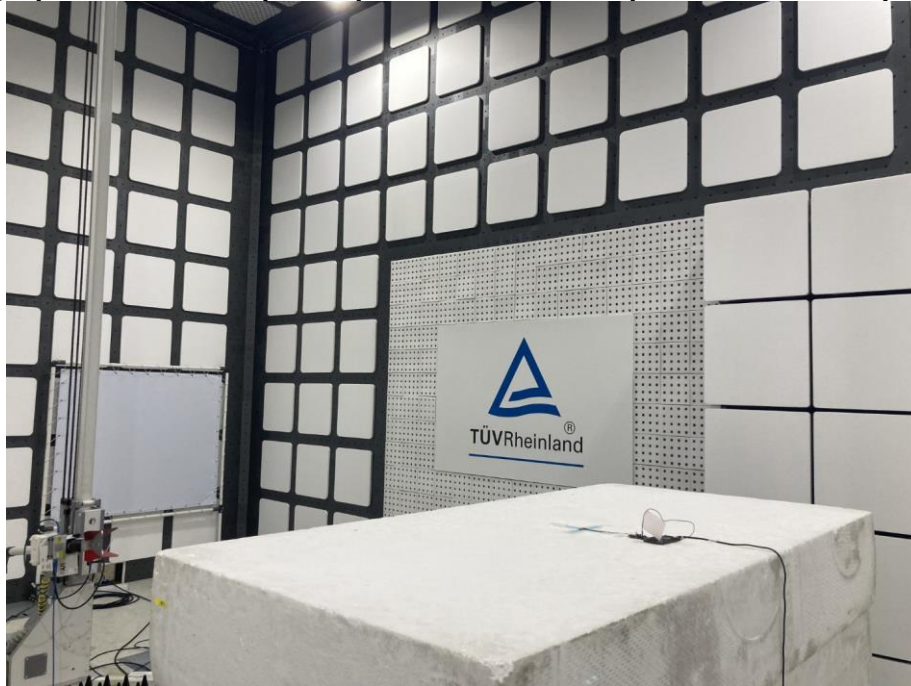
Photograph 21: Test Setup for Spurious Emissions (Back View 3, WiFi)
