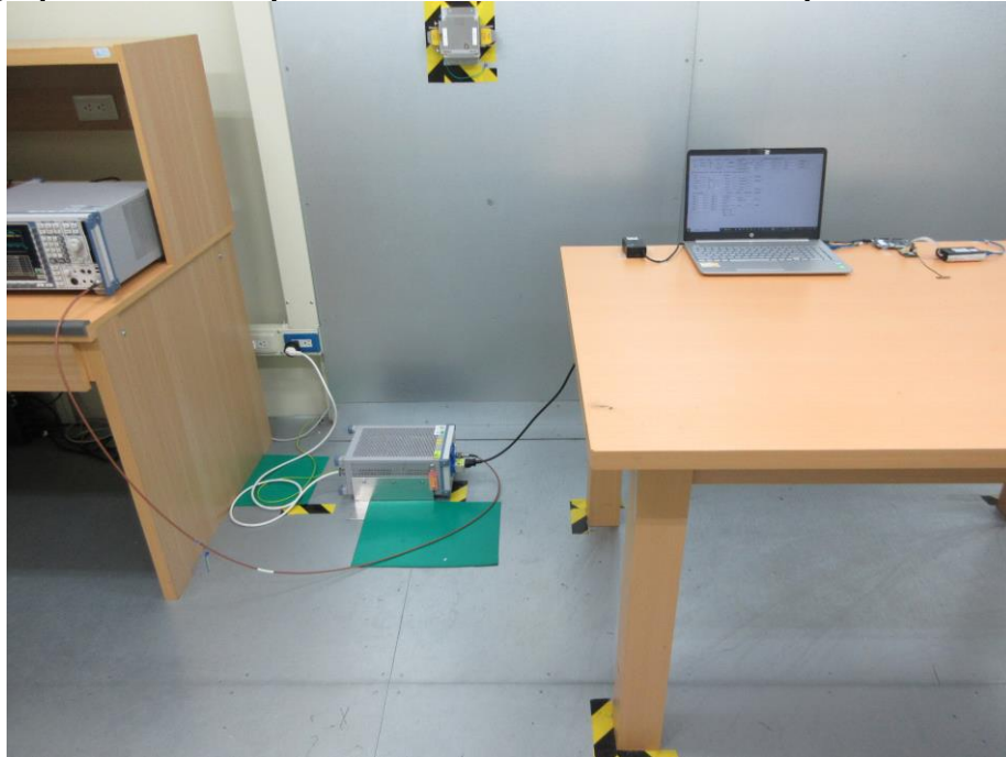
Photograph 7: Test Setup for Mains Conducted Emissions (Front View, BT)
