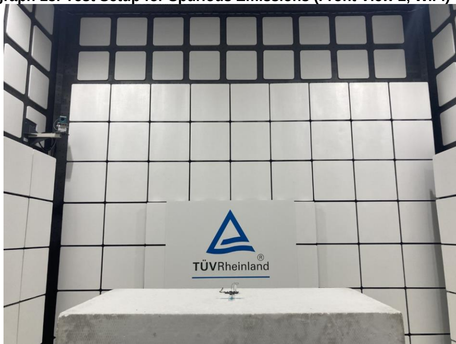
Photograph 18: Test Setup for Spurious Emissions (Front View 2, WiFi)
