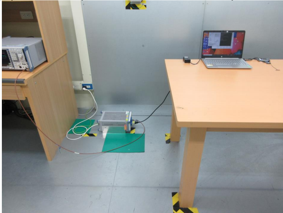
Photograph 15: Test Setup for Mains Conducted Emissions (Front View, BLE)
