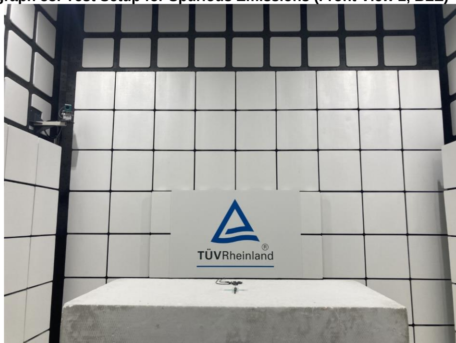
Photograph 58: Test Setup for Spurious Emissions (Front View 2, BLE)
