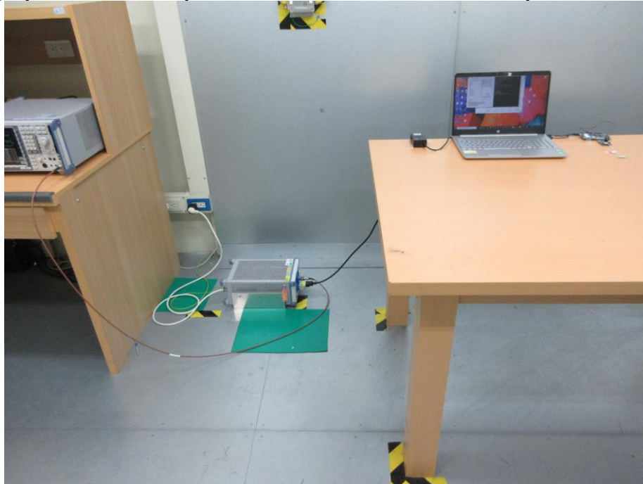
Photograph 47: Test Setup for Mains Conducted Emissions (Front View, WiFi)
