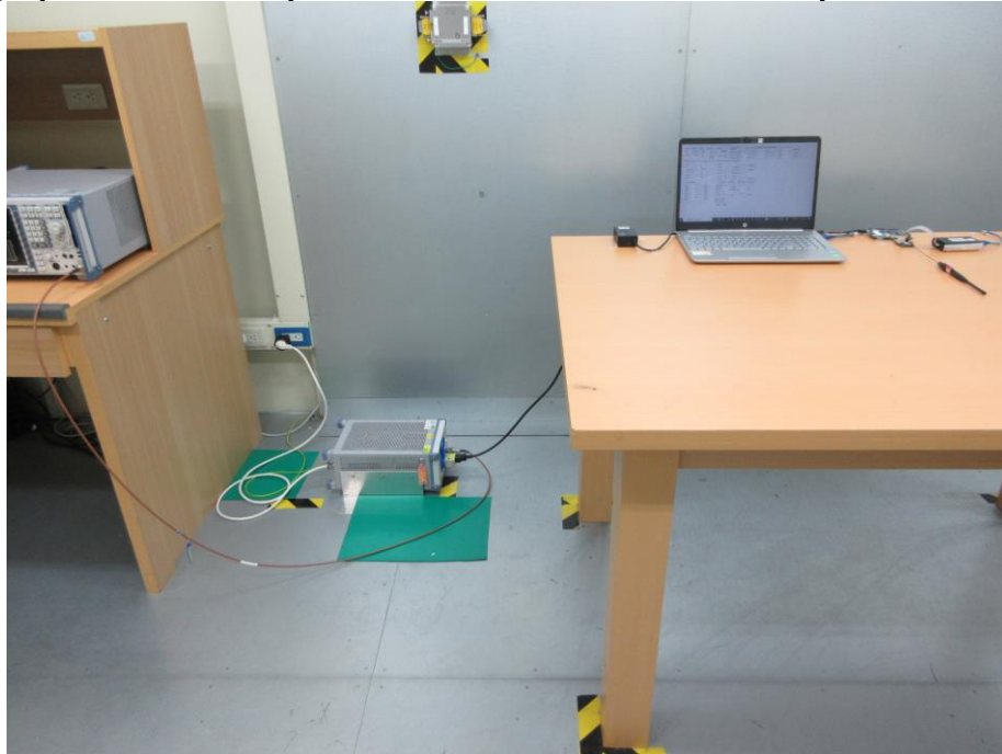
Photograph 55: Test Setup for Mains Conducted Emissions (Front View, BT)
