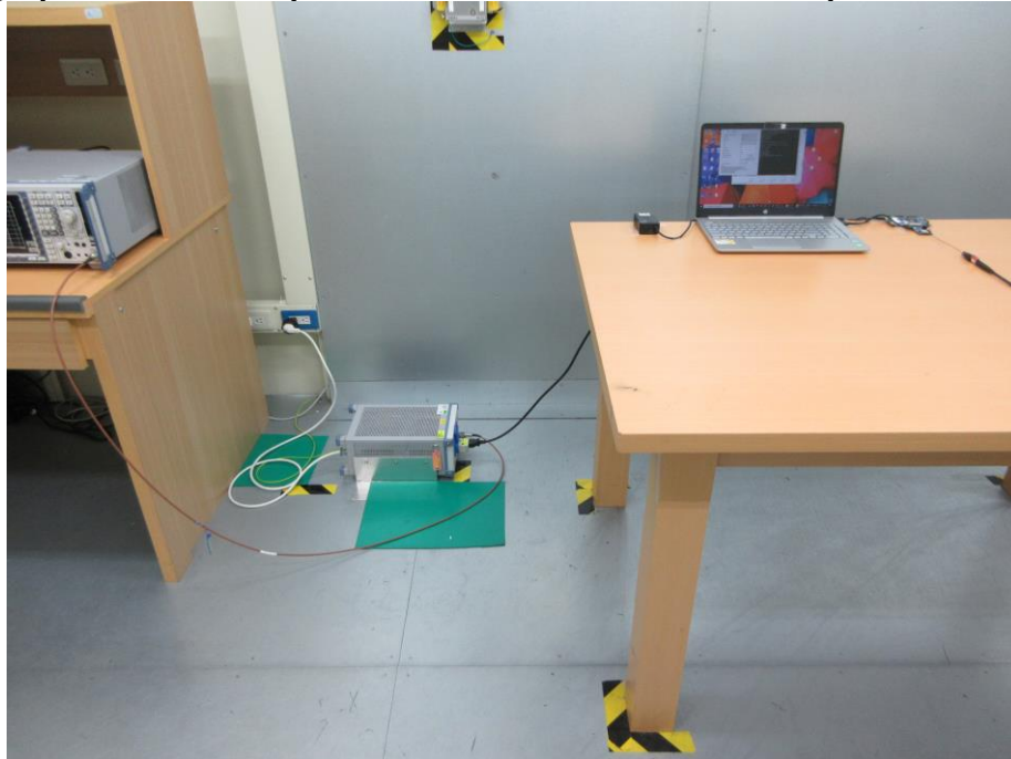
Photograph 63: Test Setup for Mains Conducted Emissions (Front View, BLE)
