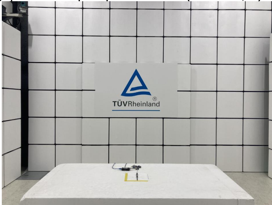
Photograph 49: Test Setup for Spurious Emissions (Front View 1, BT)
