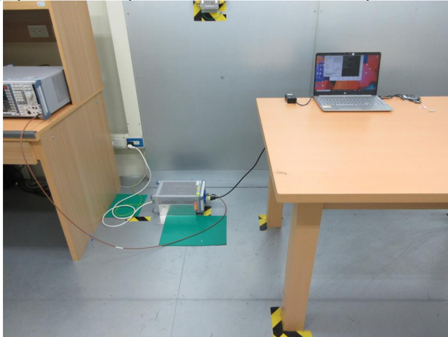
Photograph 39: Test Setup for Mains Conducted Emissions (Front View, BLE)
