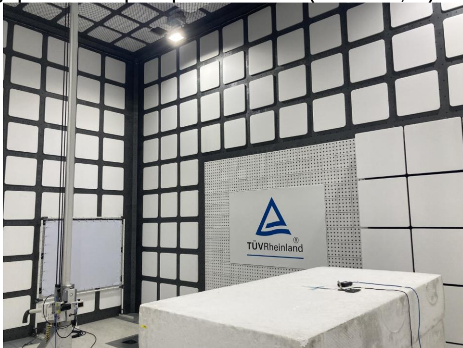
Photograph 6: Test Setup for Spurious Emissions (Back View 4, BT)
