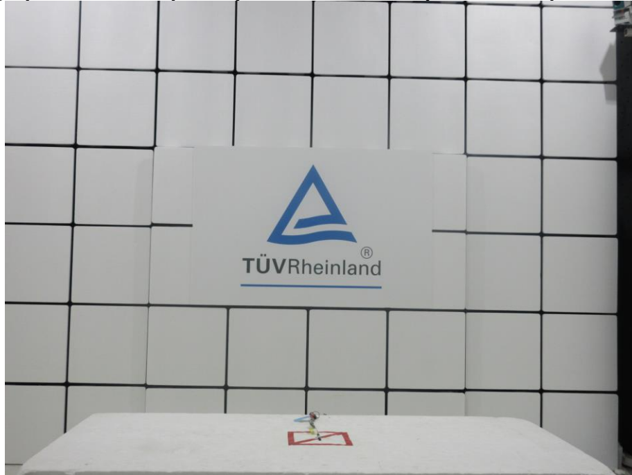
Photograph 1: Test Setup for Spurious Emissions (Front View 1)
