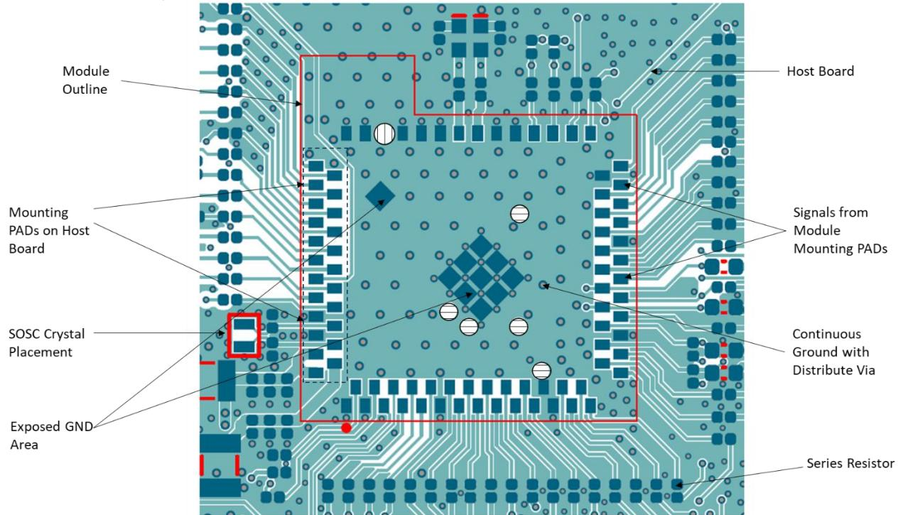
The top layer (underneath the module) of the host PCB must be ground with as many GND vias as possible.
