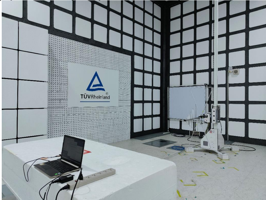
Photograph 4: Test Setup for Spurious Emissions (Back View 2, Main Source)
