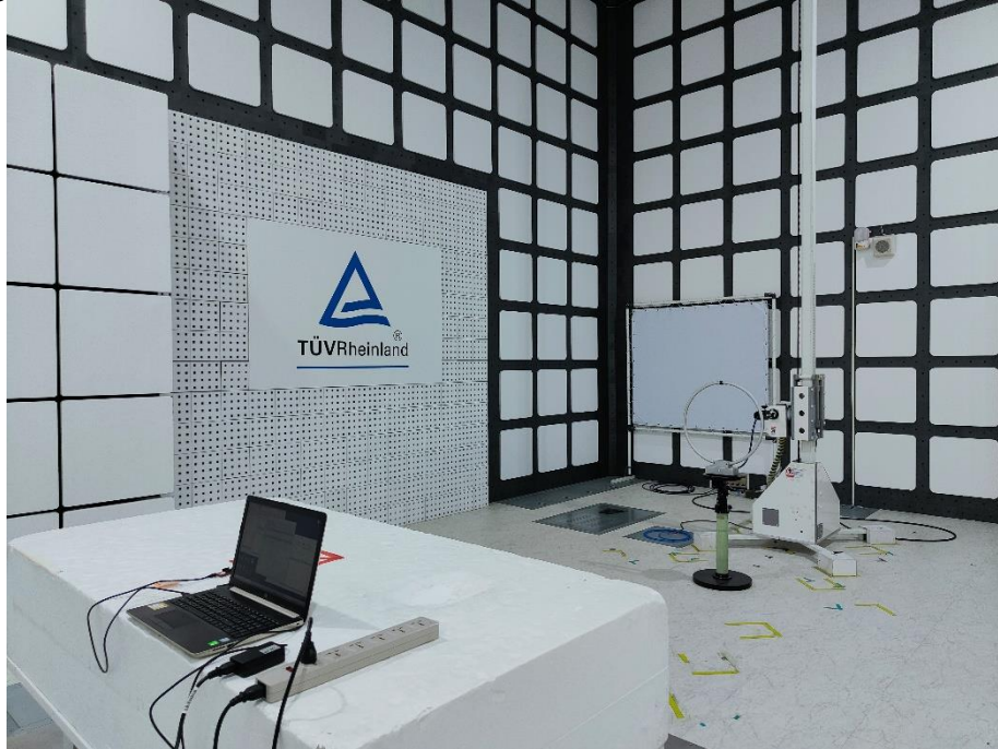
Photograph 3: Test Setup for Spurious Emissions (Back View 1, Main Source)
