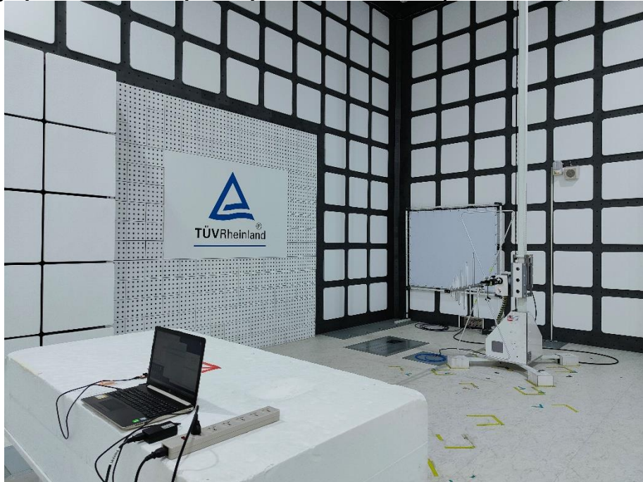
Photograph 10: Test Setup for Spurious Emissions (Back View 2, 2 nd Source)
