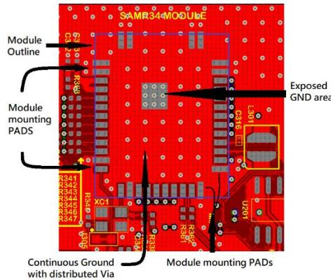
**The top layer (underneath the module) of the host PCB must be ground with as many GND vias as possible.**
