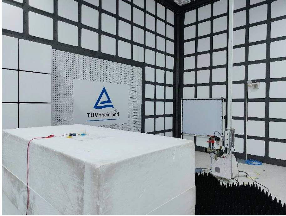
Photograph 6: Test Setup for Spurious Emissions (Back View 4)
