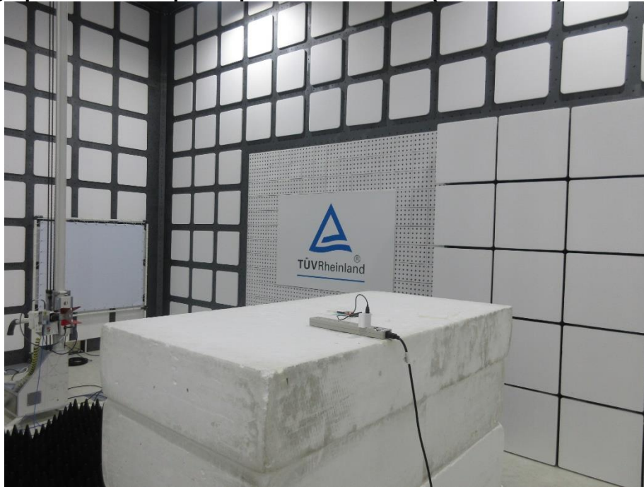
Photograph 6: Test Setup for Mains Conducted Emissions (Front View)
