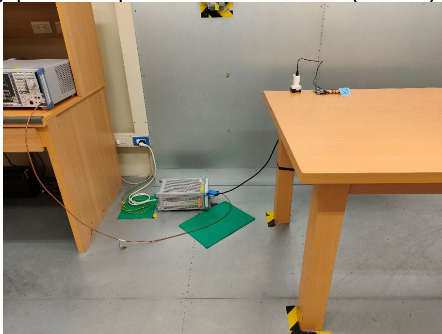
Photograph 6: Test Setup for Mains Conducted Emissions (Front View)
