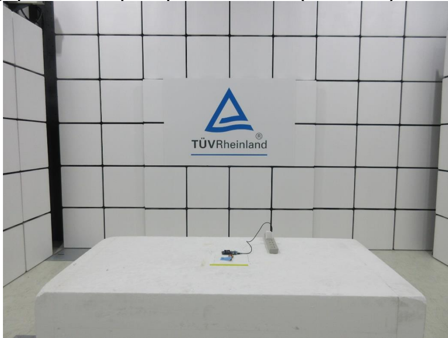
Photograph 2: Test Setup for Spurious Emissions (Front View 2)
