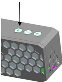
But if the system not use longer than 50 days, the system will enter the battery protection mode to protect the battery power. To resume working status, please turn off the main power switch on the right, and connect to a computer or any other standard USB port to activate it. ( see the picture as below ). When stocking it for a long time without use, please turn off the main power switch on the right, Then the system can not enter the battery protection mode.
