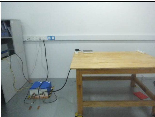
R3621-W1 Conducted Emissions Test Setup Front View
