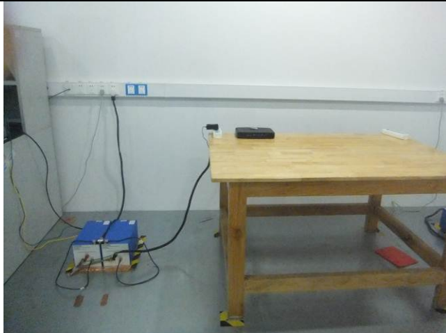
R3681-W1 Conducted Emissions Test Setup Front View
