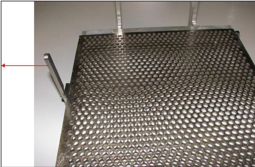
6. Lower the latch handle so it does not interfere with the print applicator. Make certain the platform is pushed against the
