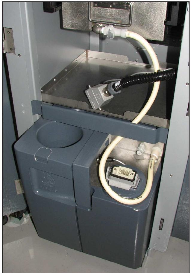
8. Press fit the hose onto the print tray connector.
