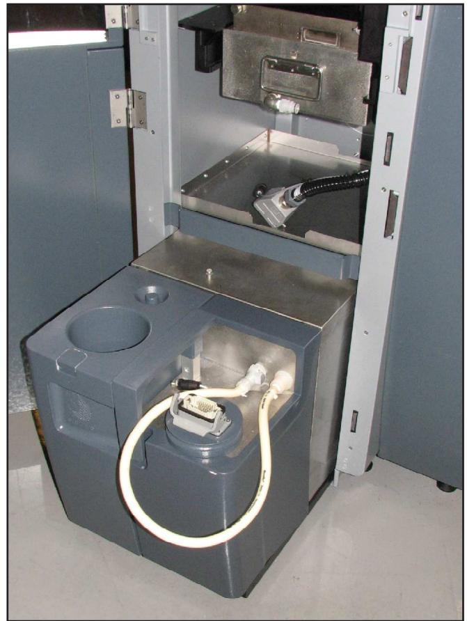
6. Press the coupling release and disconnect the material hose from the cart.
