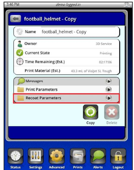
3. From here the user may open existing recoat styles and make adjustments. The user can also add recoat style ranges and sweeps to existing recoat styles.
