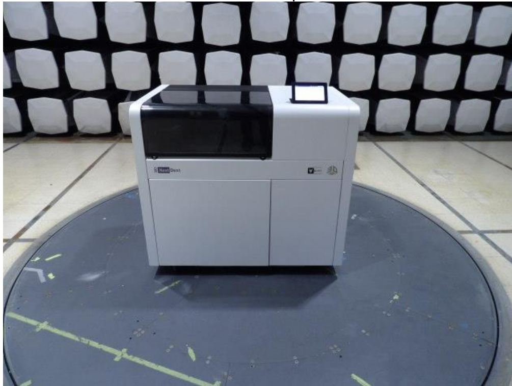
Radiated – Fundamental and Spurious below 30 MHz
