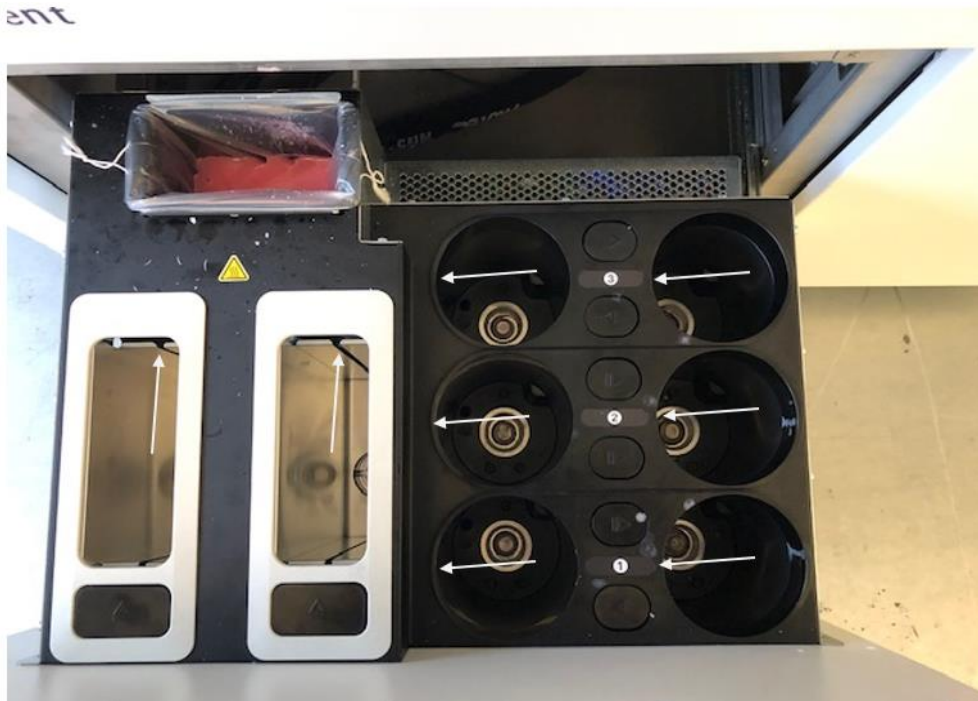
Material Distribution Module (MDM) with material bottles removed: Antenna locations are shown using arrows
