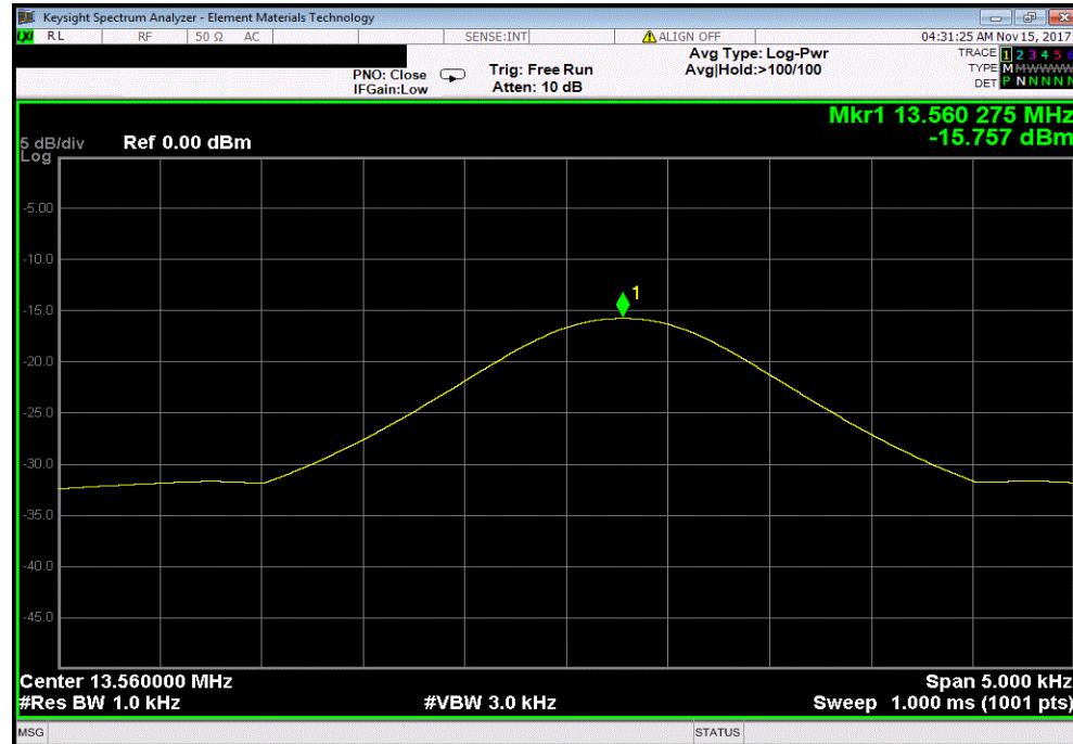
RFID, Continuous Tx, 13.56 MHz, Nominal Voltage, 24.0 VDC, +20°C
