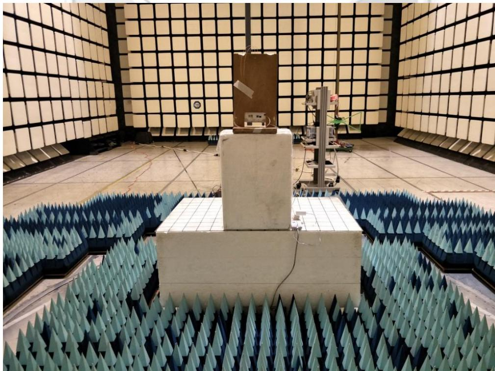
**Radiated Emissions (Fundamental and Harmonics) Test Setup (Rear View)**
