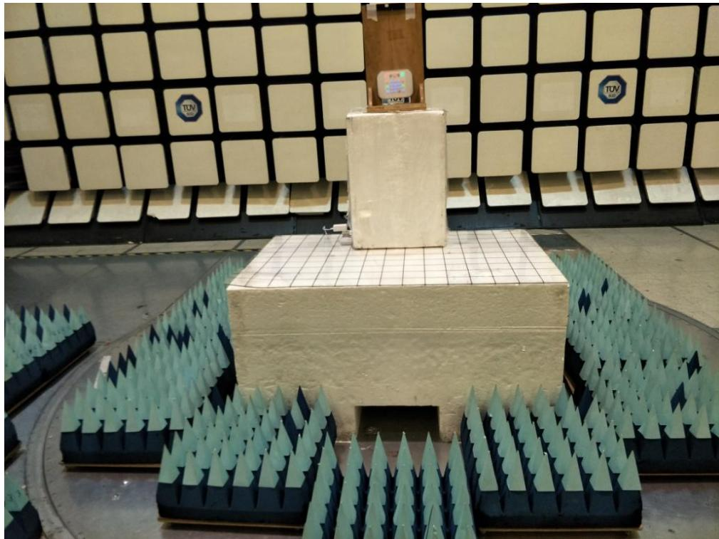
**Radiated Emissions (Fundamental and Harmonics) Test Setup (Front View)**
