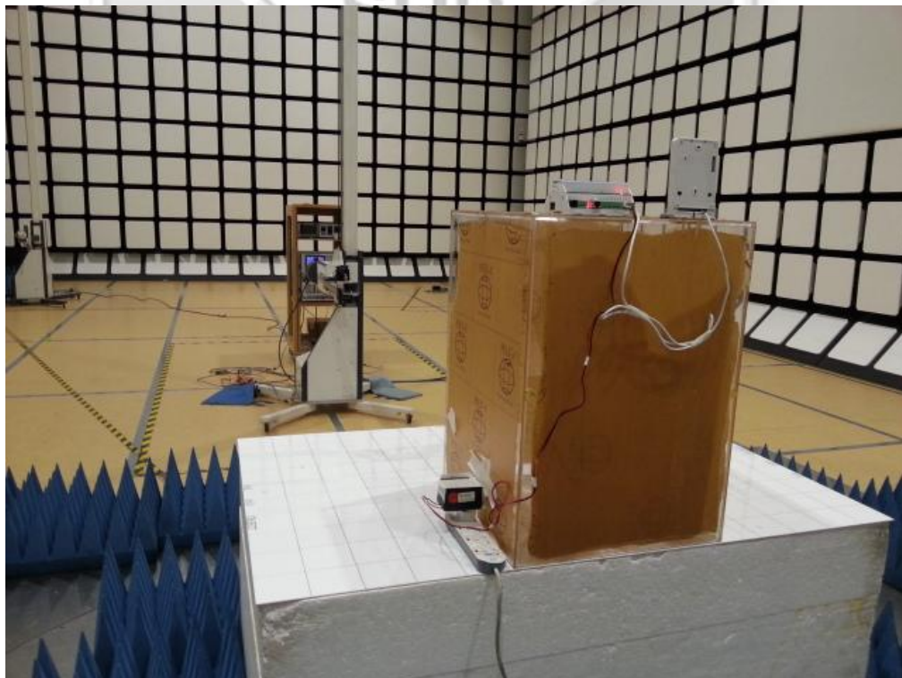
Radiated Emissions Test Setup (Rear View)
