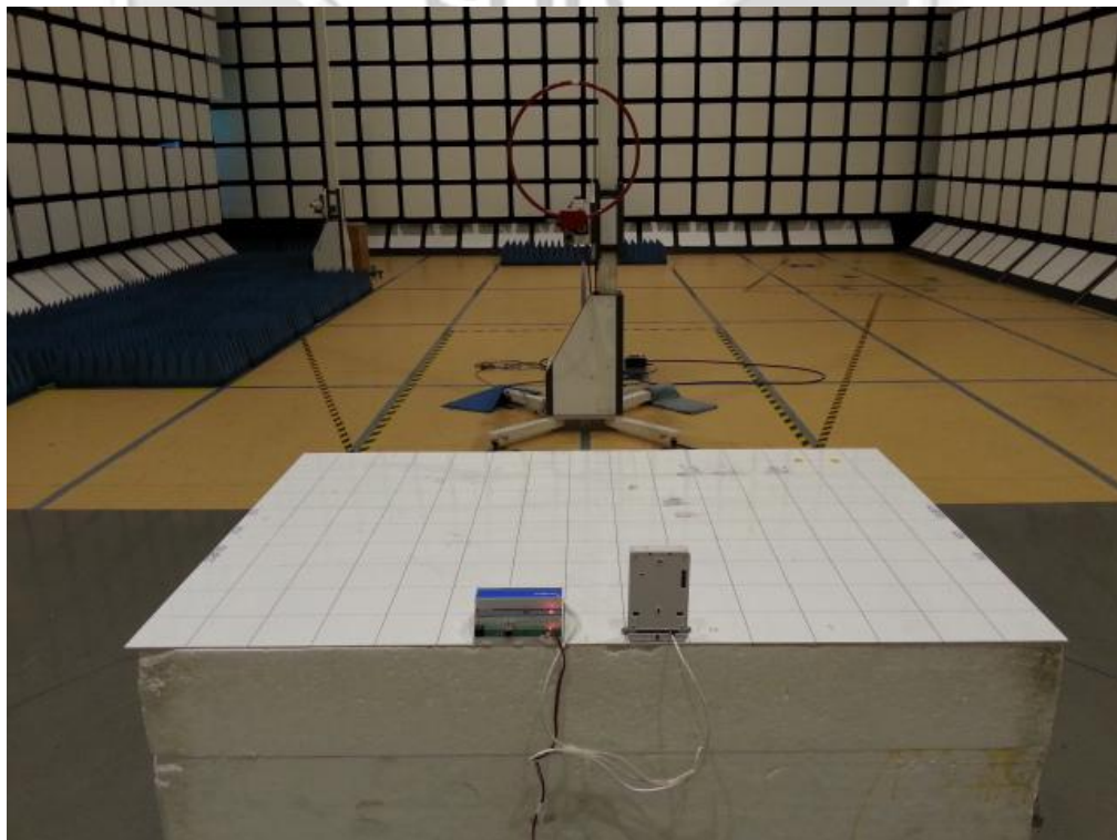
Radiated Emissions Test Setup (Rear View)
