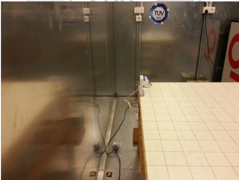
Conducted Emissions Test Setup (Rear View)
