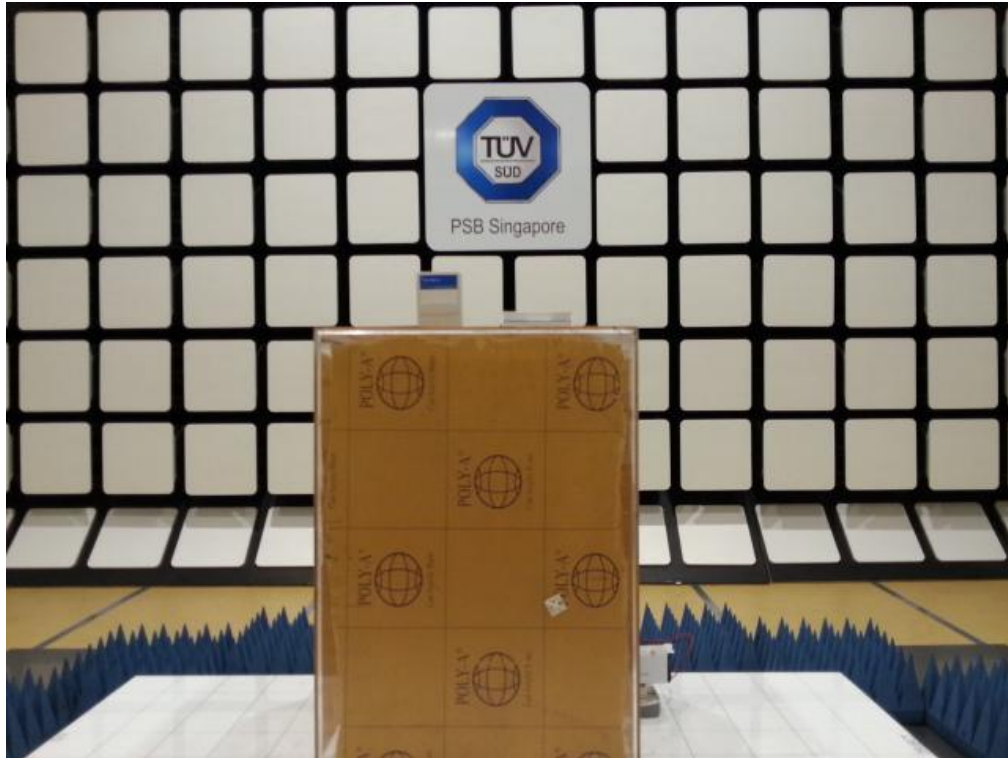
Radiated Emissions Test Setup (Front View)
