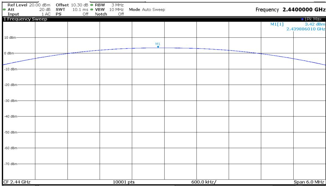
MPOP\_ch78.PNG: Maximum peak output power measured on channel 78 (operation mode 3):
