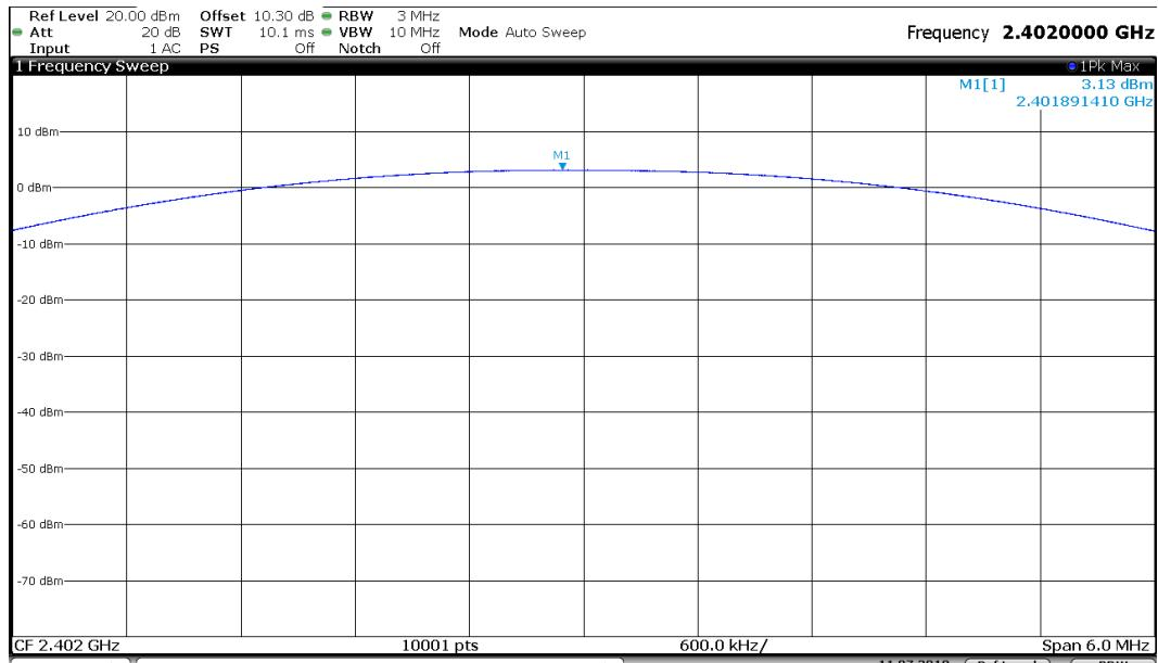
MPOP\_ch38.PNG: Maximum peak output power measured on channel 38 (operation mode 2):
