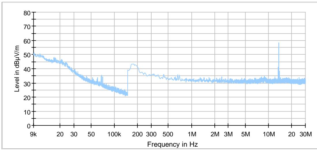
Except the fundamental of the EUT at no frequency was a value above the noise of the system therefore only a final measurement for the fundamental on the open area test site was carried out. No spurious emissions caused by the equipment under test were found.
