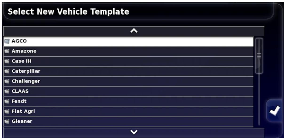
A list of pre-defined factory vehicle templates displays. Templates contain standard measurements and steering parameter information where this is available.
