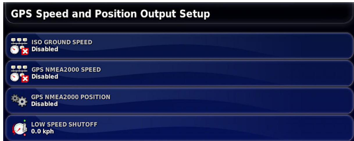
Outputs speed on ISO and/or NMEA2000 bus to the ECU.
