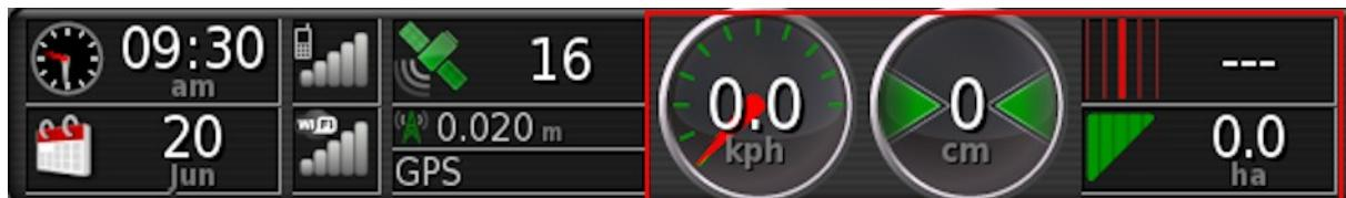
The guidance information panels may be configured to display four of six possible options: cross track error, speed, heading, swath, area worked or area remaining.
