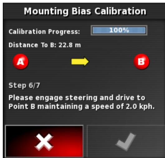
18. Stop the vehicle. Mounting Bias has been successfully calibrated.
