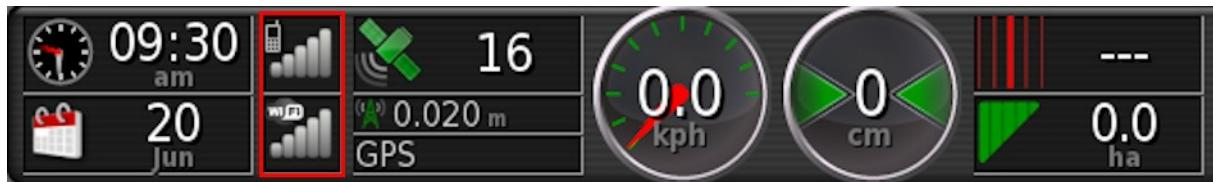
The signal strength panel shows the GPRS and Wireless signal strength.
