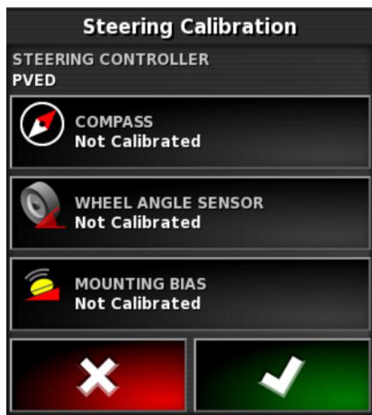
2. Select **COMPASS**. If the component reports as calibrated, still complete the calibration procedure if the receiver has not been calibrated on this vehicle.
