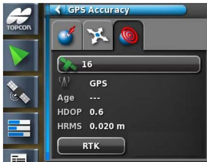
This displays the number of available satellites, the correction age (seconds) and the HDOP (lower value indicates better accuracy) and HRMS (lower value indicates better accuracy).
