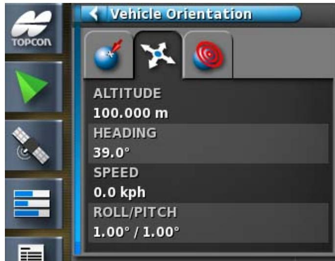
This shows altitude, heading (degrees), actual speed of the vehicle and roll/pitch (degrees).
