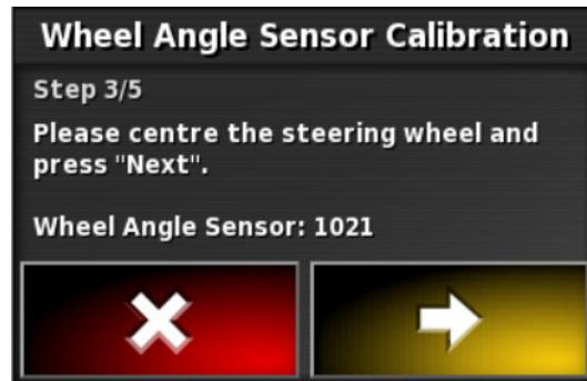
8. The system will begin to save calibration data. Wait until the screen states that the calibration is completed successfully and then confirm .
