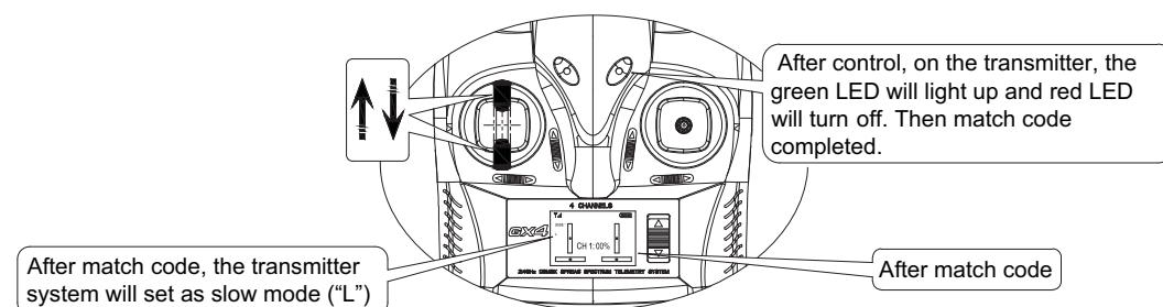
Complete the above steps, match code is finished. (The green LED on the transmitter and LED on the X6 will light up.)
