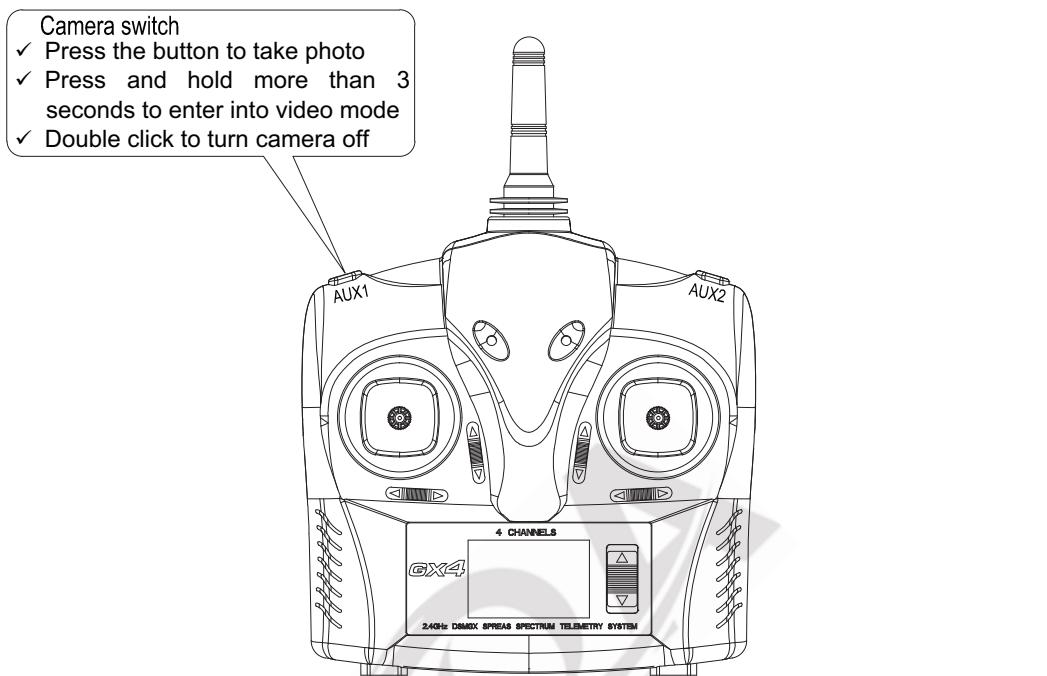
Click the "AUX1" button, transmitter has a "beep" and the camera icon appeared at LCD, it means take photo success. (Note: Press "AUX1" button once, the camera icon will appeared at LCD for one second.)
