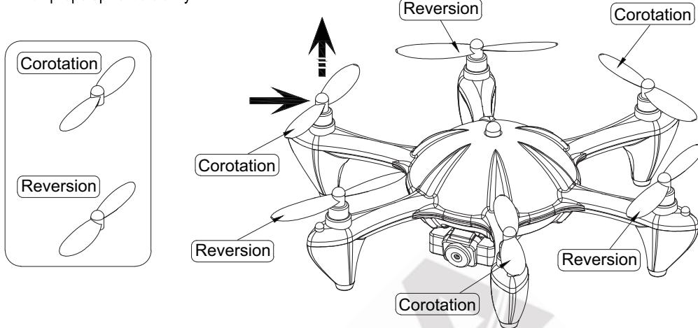
2. Position the cover's six holes with the motors. Press each of them on the motors, and then re-install the props in their correct positions on the X6.
